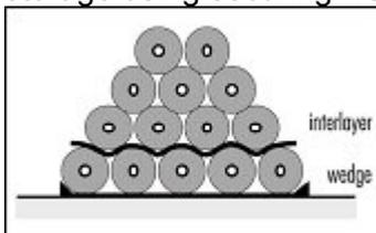
The effective weight of the upper roll layers may permanently deform the lower rolls or outer windings of the lower rolls (especially bottom rolls). The max. possible stacking height therefore depends on the weight of the rolls and the compressive strength of the foam type/grade. Trials are recommended. It may be advisable to use foam interlayer against damages.
