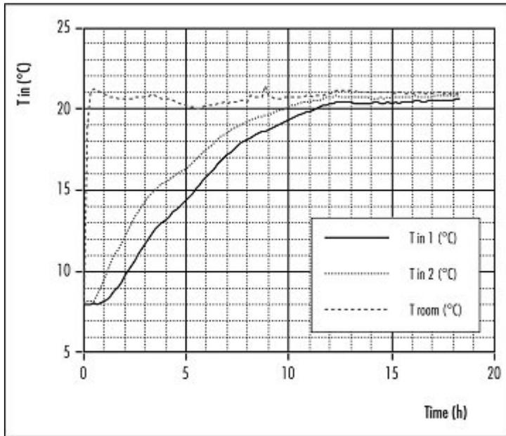
Temperature as function of time after moving a roll from 8 °C storage to 23 °C room ( $\Delta T = 15^\circ\text{C}$ ). Temperature measured at 2 different locations inside the roll windings.
